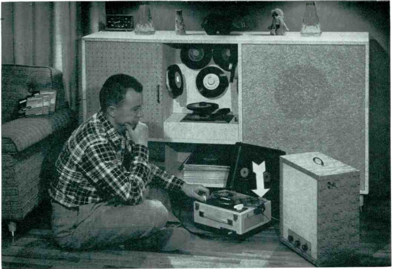
Fig. 1: Whether recording live, from TV or FM, or just dubbing records as shown here, it's often a distinct advantage to hear what you are recording as you record it. Even with an inexpensive home recorder, the addition of an auxiliary tape head (at arrow) and separate playback system make this easily possible.
