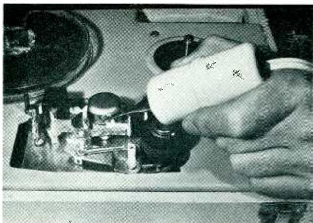
Fig. 6: Demagnetizing your tape head(s) should be a regular procedure every ten hours or so. It's the only way to be certain that accumulated residual magnetism is dispelled before it starts erasing the high frequencies of your already recorded tapes. And incidentally, erasing those same high frequencies on the test tape, ruining it.
