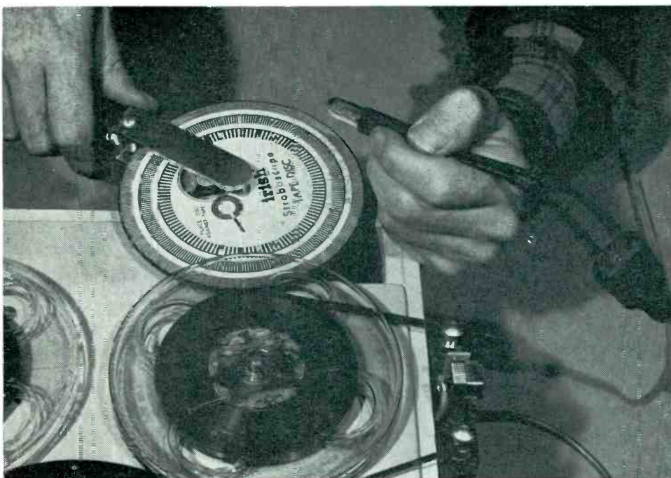
Fig. 9: The stroboscope tape disc, when held against the surface of the moving tape, will revolve at the same speed as the tape and thus indicate the tape speed. First measure the speed of the tape in the recorder in the regular manner, then pass the tape around the auxiliary head and check again. The two speeds must match!
